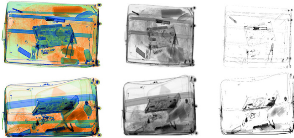
Figure 1 A sample image containing a steel barrel bores (top left cylinder in the top row) from the baggage dataset. The left image (in both rows) is the raw dual view x-ray scan, in the middle, the grey scale smoothed one, and on the right, the b/w thresholded one.
