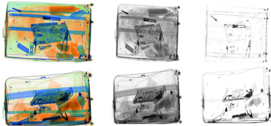
Figure 4.18: A sample image containing a steel barrel bores (top left cylinder in the top row) from the baggage dataset. The left image is the raw dual view x-ray scan, in the middle the grey scale smoothed one, and on the right the b/w thresholded one.
